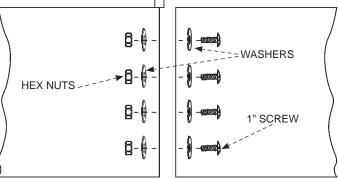
Attach two long posts to the corner of the deck closest to the pool using the 2" screws and hex nuts as shown in Close Up 3.
